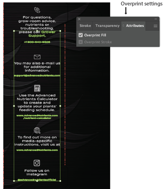
Green type is set to Overprint - the overprint setting for the green type is shown in Attributes.
