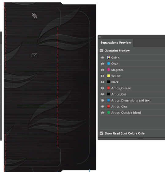
Overprint Preview ON shows how the artwork will print. The white and green type disappear because of the overprint setting.
